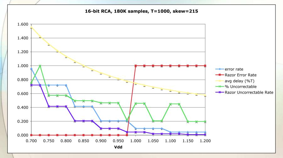
Razor only works in size T window 100% False Razor-induced errors when min < skew Must turn off Razor and accept some level of error Many uncorrectable errors when T+skew not large enough
