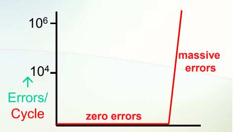
Increase Clock Frequency → Or Decrease Supply Voltage Or Increase Aging Degradation Or Increase Process Variations
